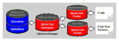
The BEACON development package provides a seamless framework for generating and unit testing software from Simulink and Stateflow models. The generated software can be executed on a variety of platforms, including production ECUs.
