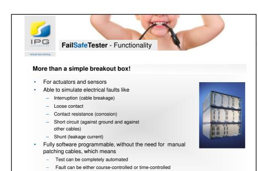
Complete test configuration can be stored and re-loaded
